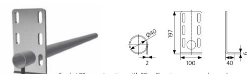
Bracket 8891 can together with 8890 Pipe ø40x2000mm be used to assemble ploughs Maxi 8800, Maxi foldable 8800-VF and Plough heavy duty 2800 to the conveyor frame.
