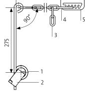
Holder H and Spring lever 9178 are used in most of Vendigs belt cleaners. For larger belt-widths the bracket Holder HD and two spring levers are used. Detailed installation instructions are included with all belt scrapers.
