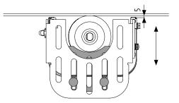
Its openings are maximized according to the enquirements of the norm in order for reurn material to fall through. When the safeguard needs to be opened, open the two screws to swing open the guard that will stay in place in the onesided hinges.
