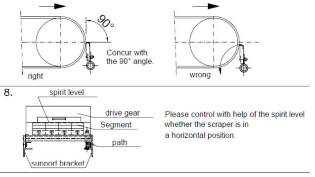
When it is secured, that the scraper is aligned according to position 7 + 8 weld the brackets at the chutes (construction, chute)
